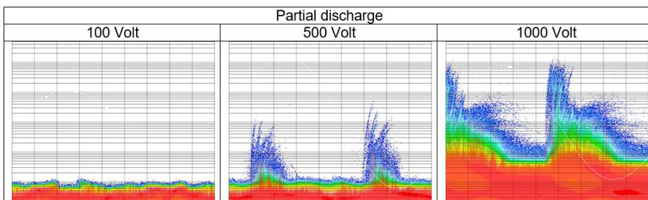
However, the discharge of a cavity can also lead to several discharge structures (fingers). This depends on the geometry, field distribution, permittivity and other factors. The cavity discharges take place at the greatest voltage change. The consequence of this partial discharge is a slow but
